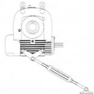
**Shaft Mounted Unit with Torque Arm**
